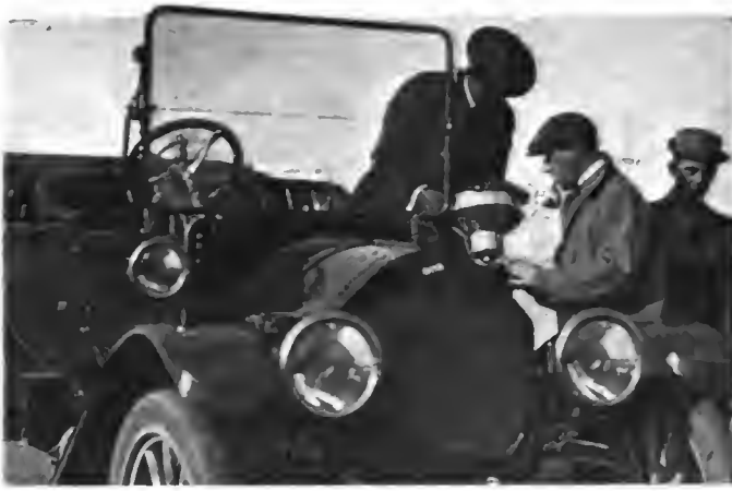
Filling special fuel tank in Harroun carbureter test
